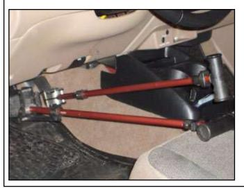
Peddle Master is designed to give disabled people the ability to drive their vehicles on their own. As long as they have access to a vehicle with an automatic transmission, they can get behind the wheel and hit the road. The Peddle Master can control the brake and gas pedals, and it's affordable and easy to transport.
